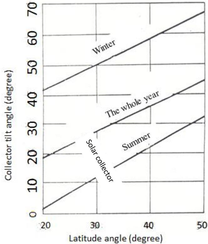
Figure (4) relation between the collector tilt angle and the latitude angle
