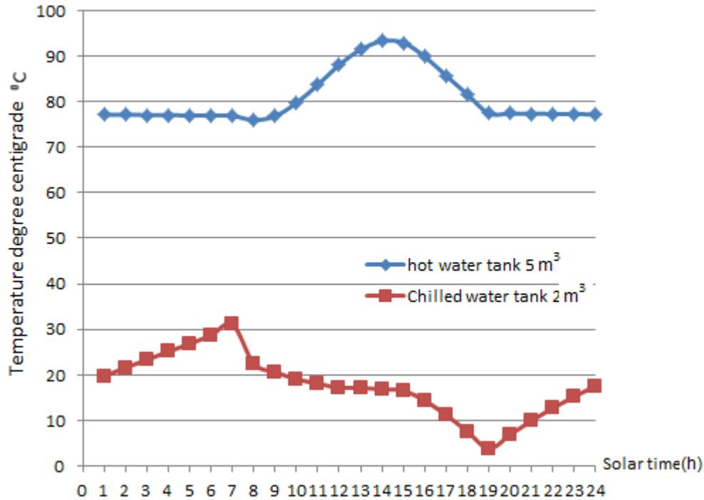
Figure 7. Temperature of hot and chilled water tanks for a single-glazes collector
