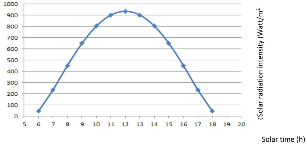
Figure (5): Incident radiation on the collector at the design day for the cooling system
