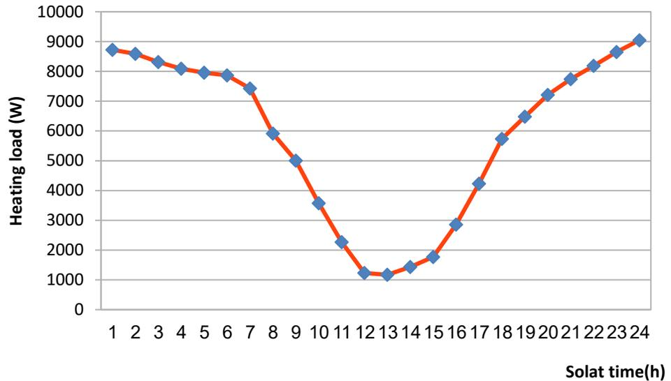
Figure (2) Heating load during design day
