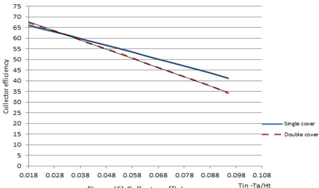
Figure (6) Collector efficiency curve
