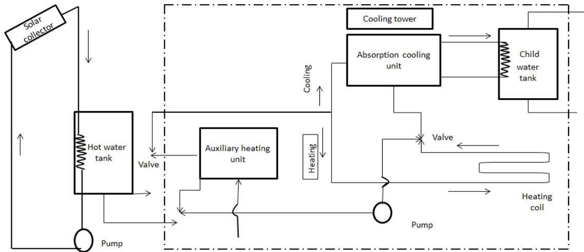
Figure (3) Solar powered heating and cooling system
