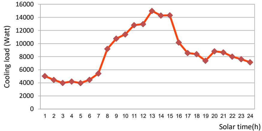
Figure (1) Total cooling load
